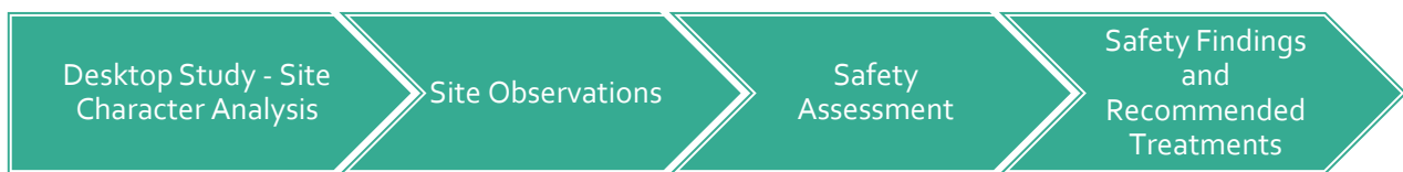
Figure 2: Post Construction Safety Assessment Process
