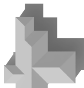
Combination Gable And Hip Roof
