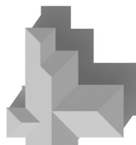
Combination Gable And Hip Roof
