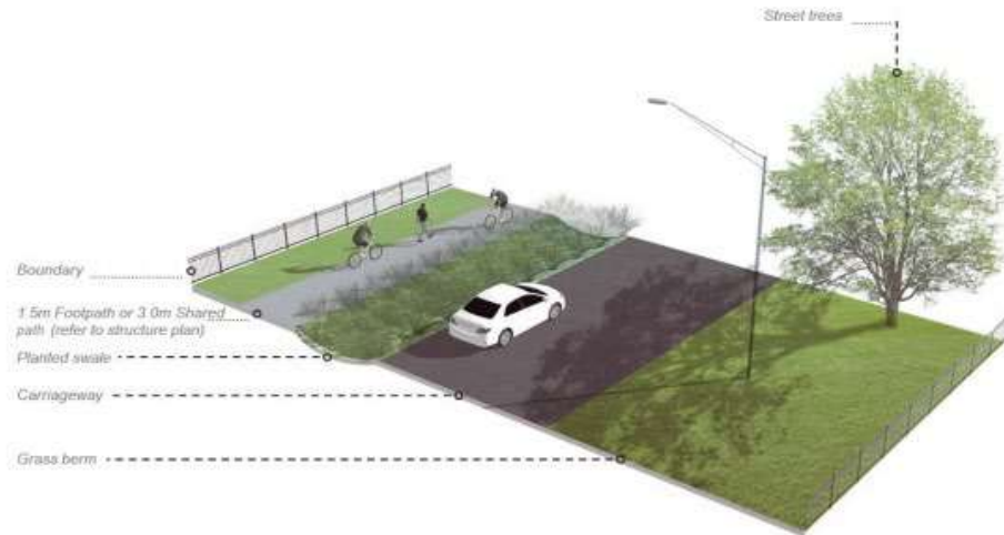
Example image. Typical 18m street with separated 3m shared cycle path or 1.5m footpath (refer structure plan) and vegetated drainage swale
