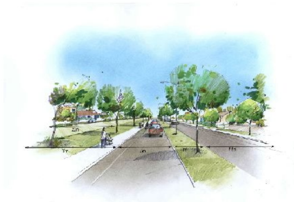
Figure 1: Cross section through Victoria Road showing the swale separating this main road from residential development to the East.
