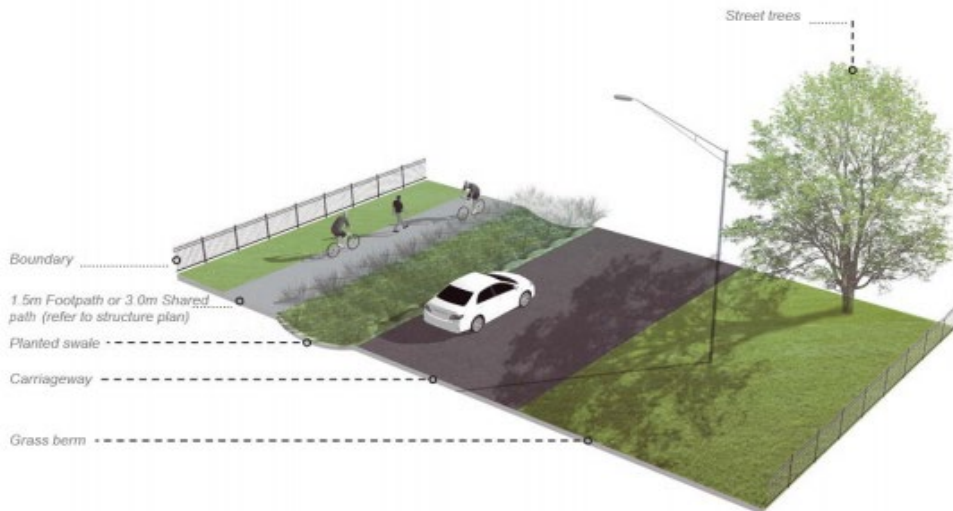
Example image. Typical 18m street with separated 3m shared cycle path or 1.5m footpath (refer structure plan) and vegetated drainage swale
