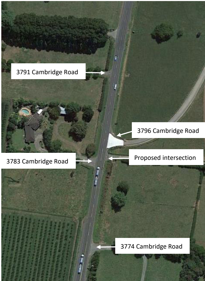
Figure 13: Access separation distances
