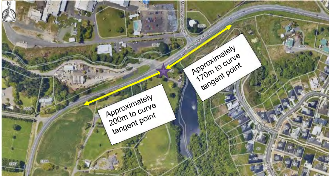
Figure 16: 3838 Cambridge Road Access (purple star = vehicle crossing)
