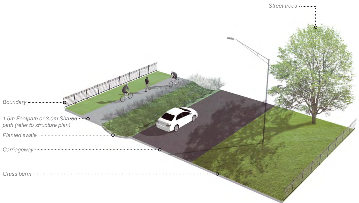
Example image. Typical 18m street with separated 3m shared cycle path or 1.5m footpath (refer structure plan) and vegetated drainage swale.
