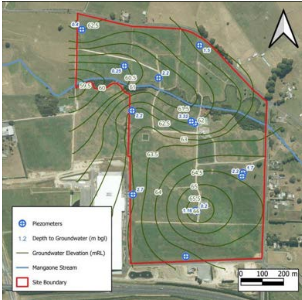
FIGURE 5: INFERRED GROUNDWATER LEVEL CONTOURS (BECA, 2023)
