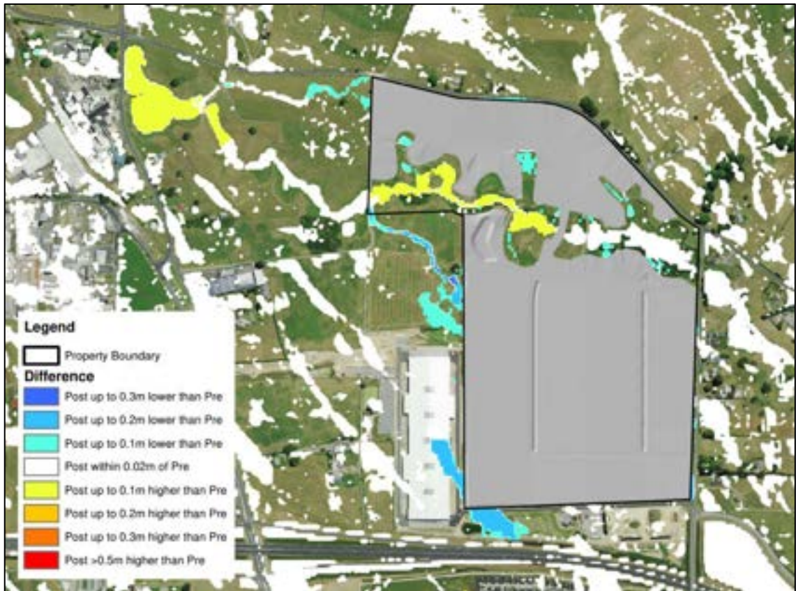
FIGURE 13: FLOOD LEVEL DIFFERENCE FOR 1% AEP STORM EVENTS
