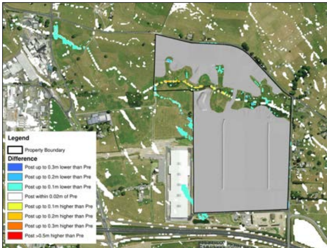
FIGURE 15: FLOOD LEVEL DIFFERENCE FOR 50% AEP STORM EVENTS
