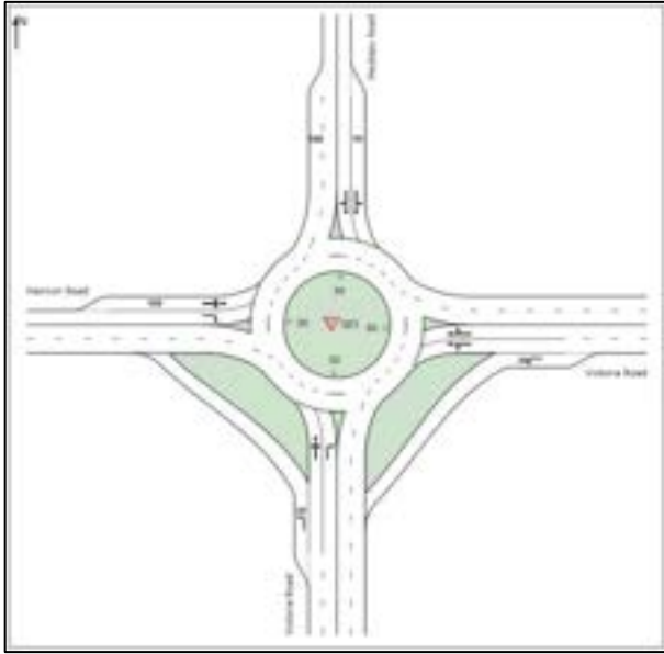
Figure B-13-3: Configuration assessed in the HG ITA for the future Victoria Road/ Hautapu Road roundabout
