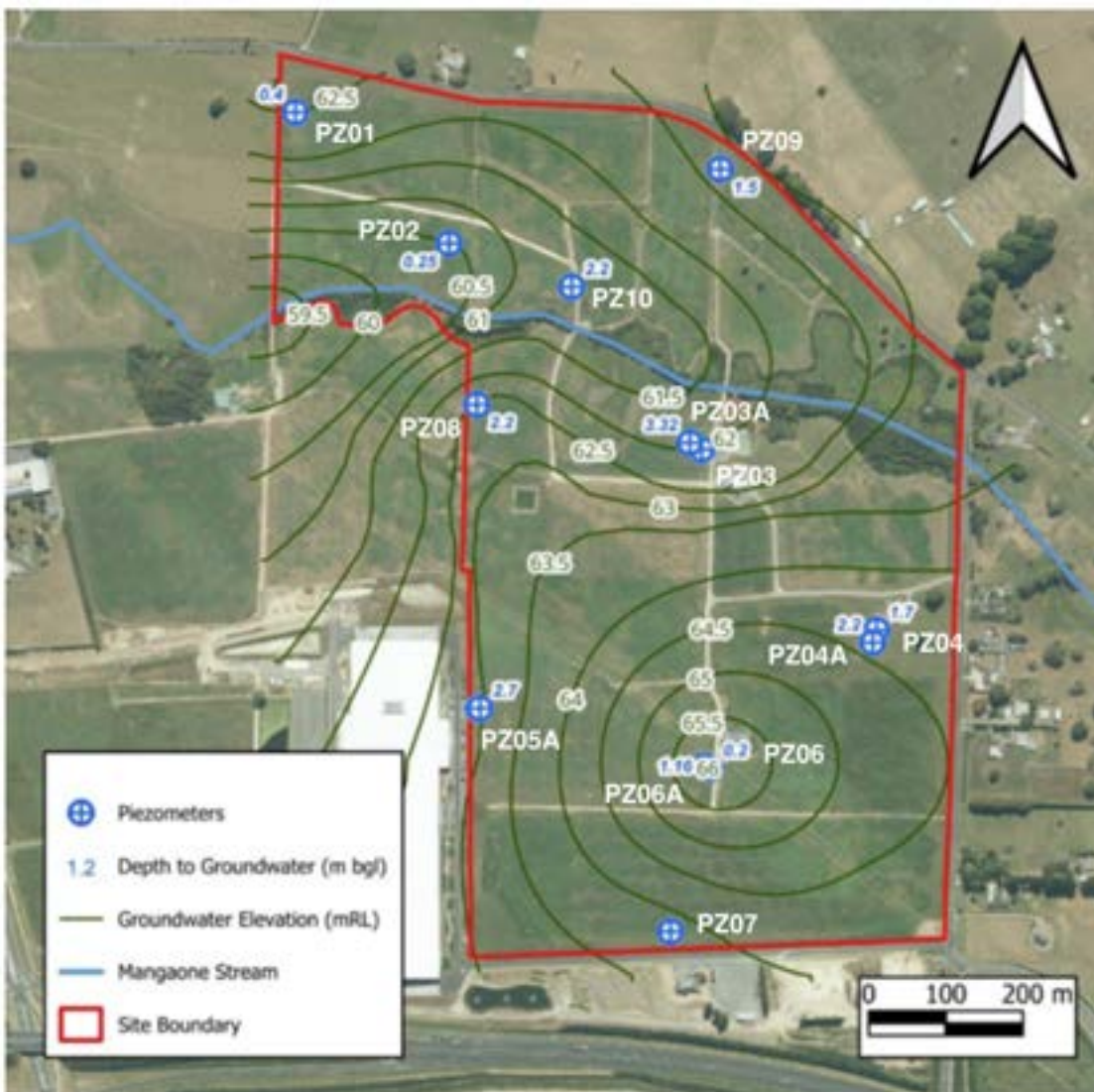
Figure 4: Inferred Groundwater Level Contours; where piezometer monitoring indicates perched levels, the shallowest (highest) water level is shown.
