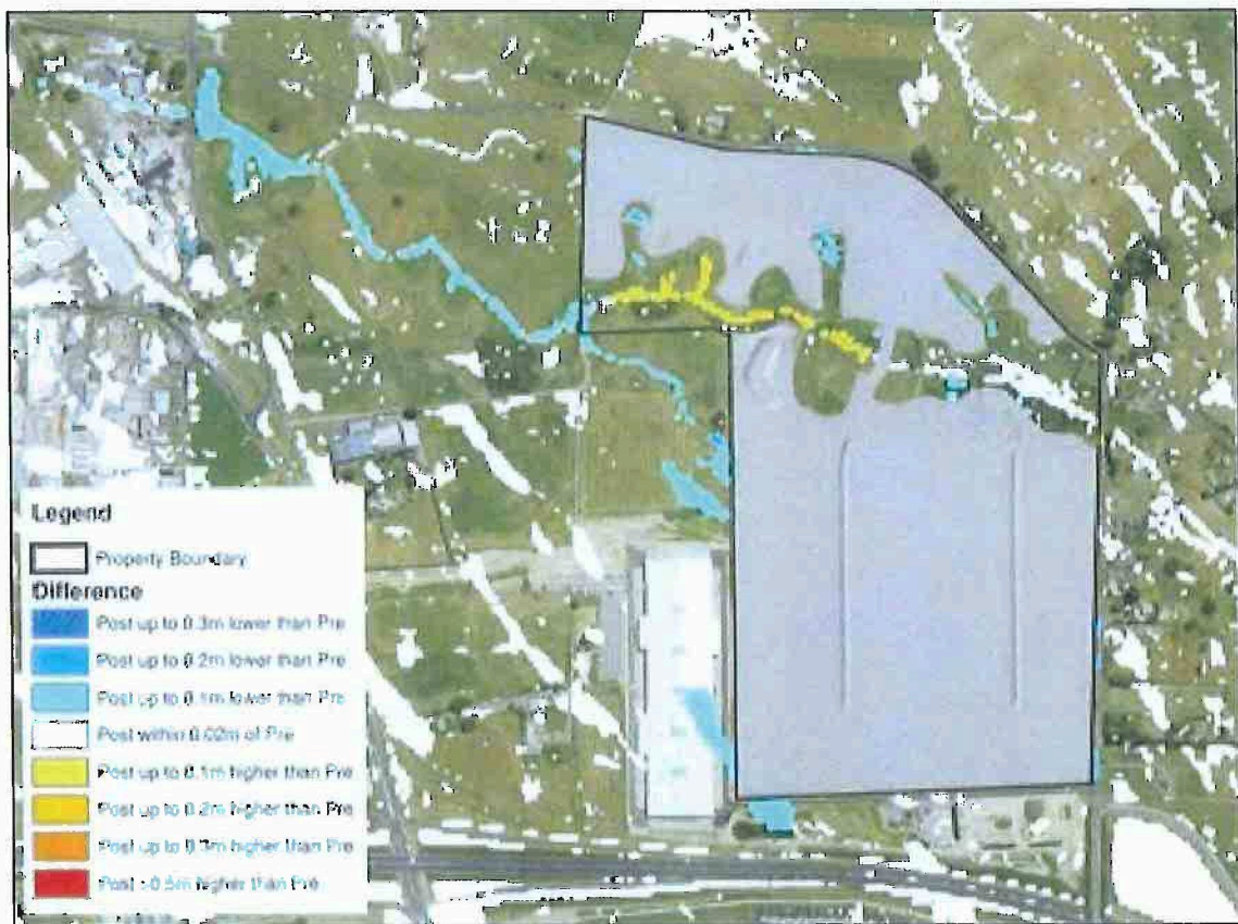
FIGURE 14: FLOOD LEVEL DIFFERENCE FOR 10% AEP STORM EVENTS
