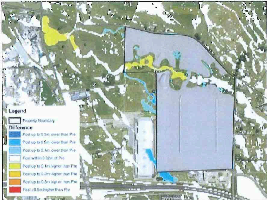
FIGURE 13: FLOOD LEVEL DIFFERENCE FOR 1% AEP STORM EVENTS
