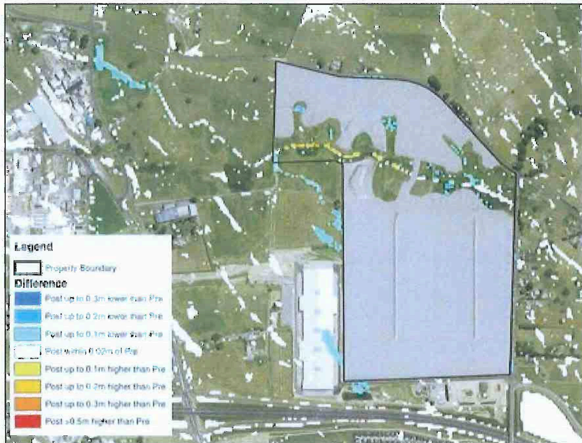
FIGURE 15: FLOOD LEVEL DIFFERENCE FOR 50% AEP STORM EVENTS
