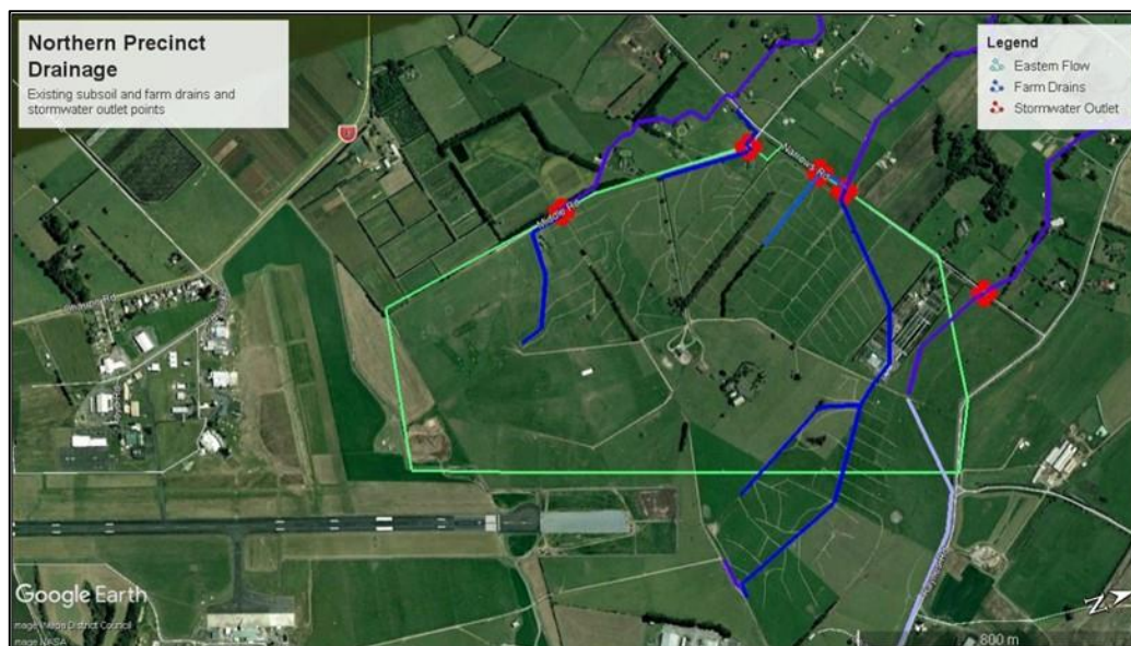
FIGURE 3: EXISTING FARM DRAINS, OUTLET POINTS AND SUBSOIL DRAINS WITHIN THE TPL BLOCK
