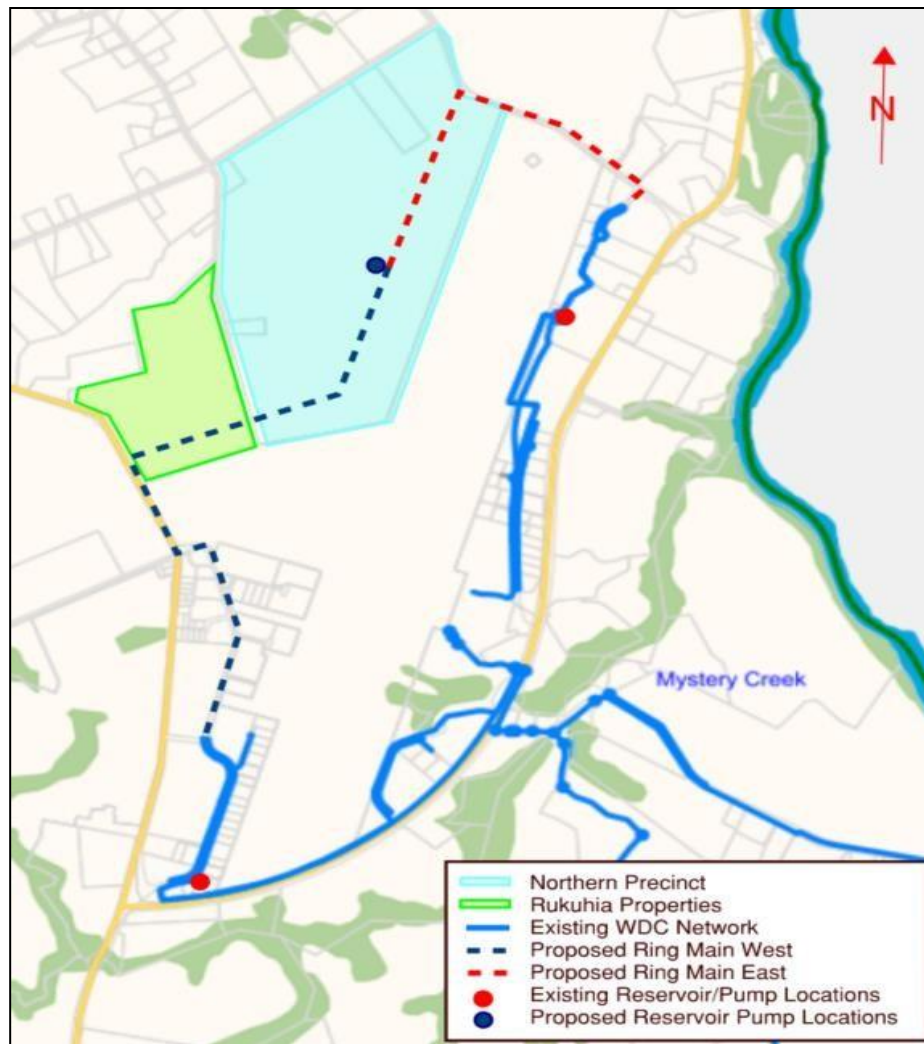
Figure 2 - Existing and Proposed Water supply
