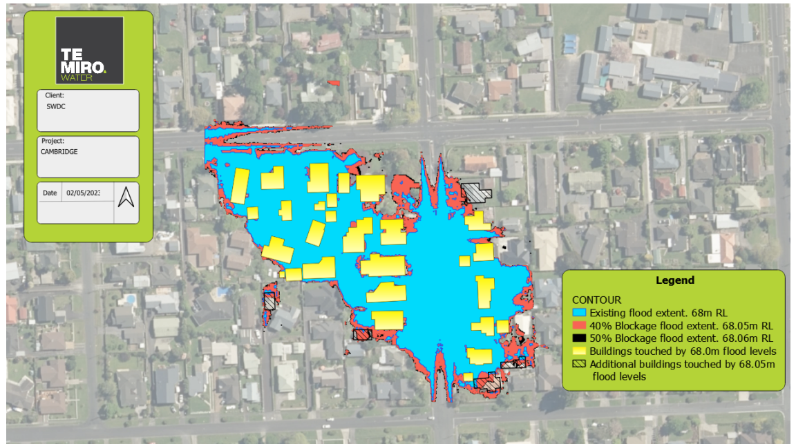
Figure 6. Buildings affected by ponding.
