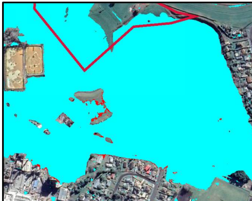
Figure 4.3 – HGL along site boundary along Mangapiko Stream – 100-year storms
