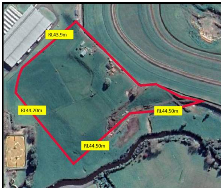
Figure 5.1– Minimum finishes floor levels through the site
