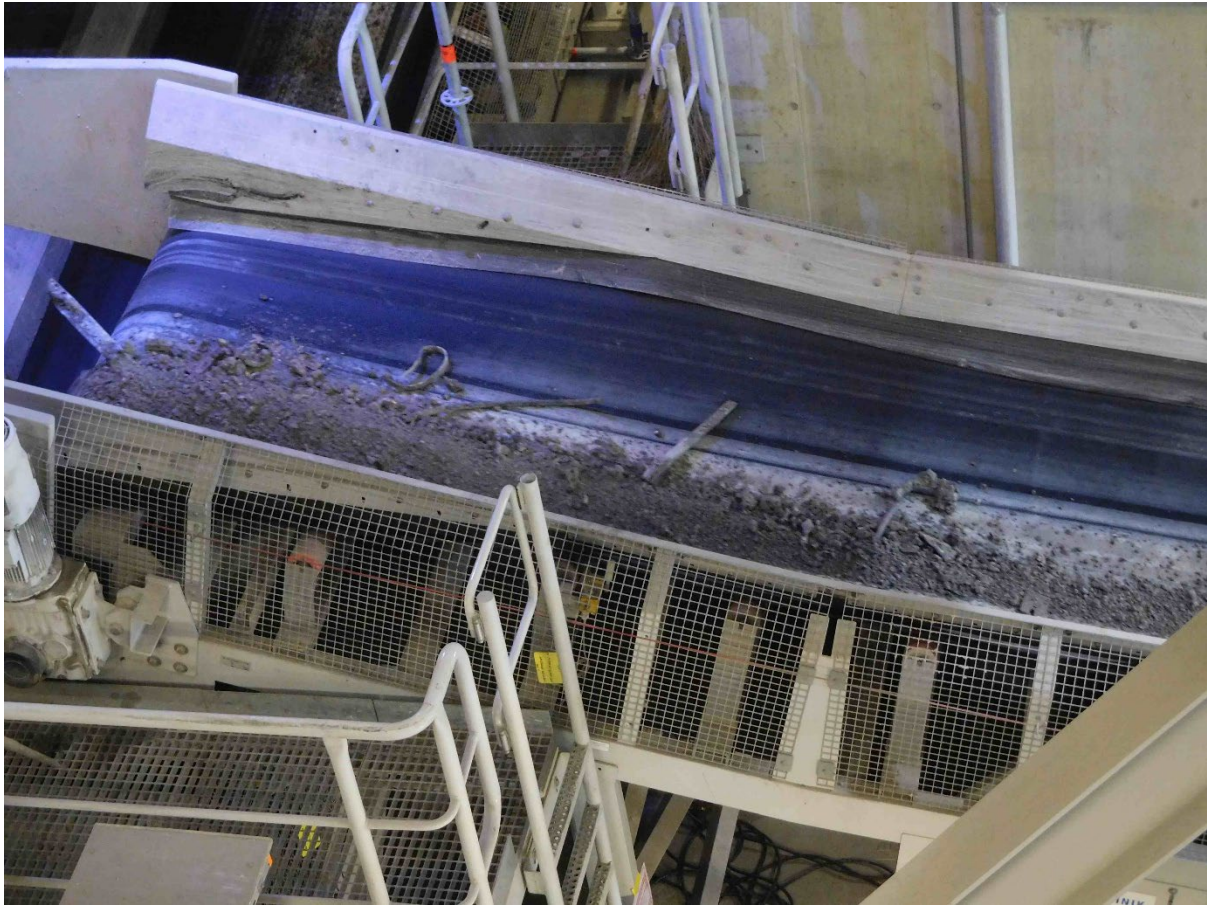
FIGURE 3 - FERROUS METAL IN BERN BOTTOM CLINKER FOR RECOVERY
