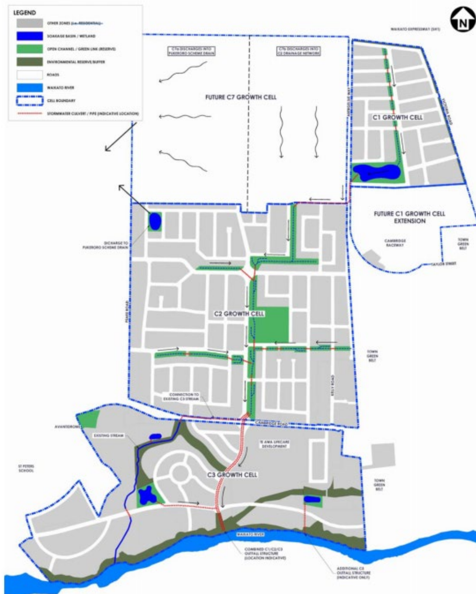
Figure 9: Proposed schematic stormwater layout for the C1 and C2/C3 Growth Cells (also showing future growth cells C7 and C1 Extension)
