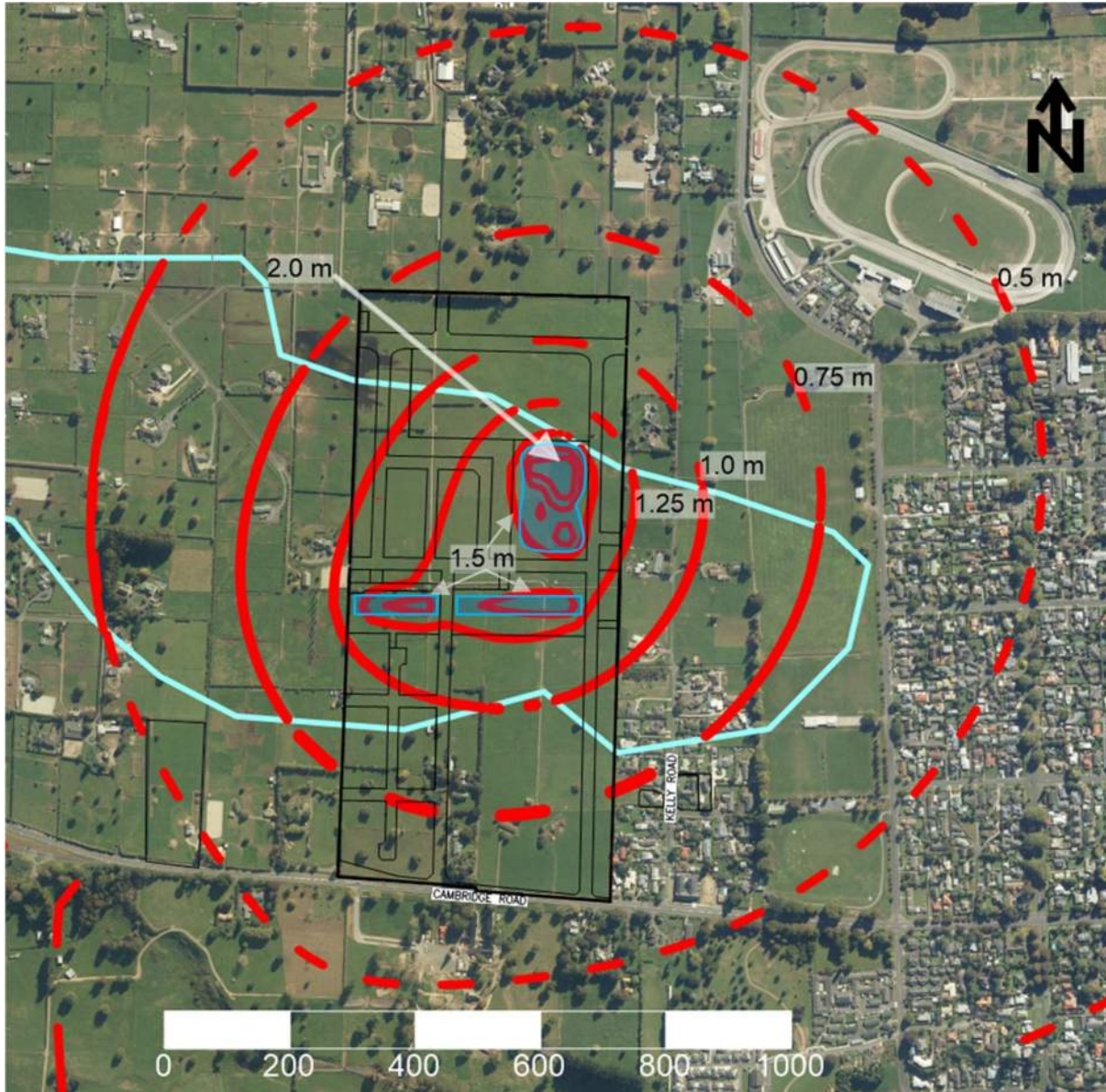
Figure 8: Close up of calculated drawdown contours (0.25 m intervals) from long term operation of soakage basin and stormwater swales. Drawdown contours are dashed beyond the known extent of the iron pan (outlined in light blue and consistent with areas identified by BTW as having a deeper, if any perched level) to note the much lower risk of measurable drawdown eventuating in these areas. Excavations demarcated by blue rectangular polygons.
