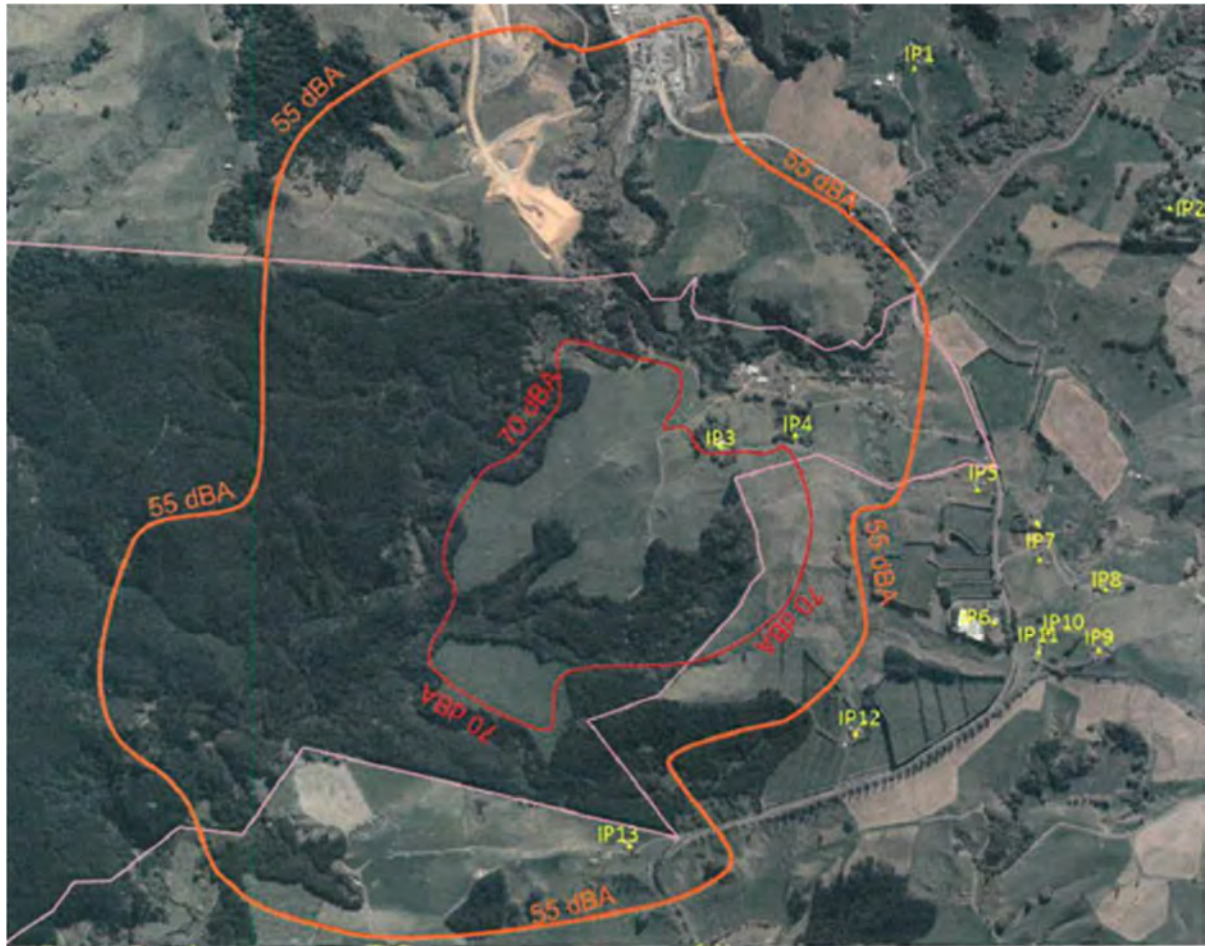
Figure 18: Predicted L_{Aeq}(5 \text{ minute}) sound pressure level contour (55 dBA and 70 dBA) taken from Noise Assessment prepared by Cardno
