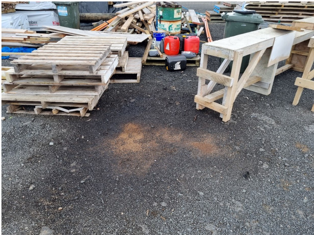
Photograph 4: Staining on ground next to minor fuel, oil and chemical storage in Livingstons Construction yard (southeast of the site) (Feature of interest 2).
