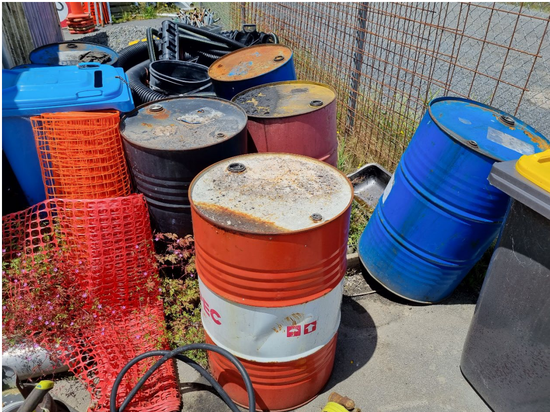
Photograph 18: 200L Steel drums (empty to half full - containing kerosene and engine oil) behind dangerous goods storage container. 5 within a wooden 'bund' and 2 outside of bund on asphalt (Feature of interest 14).
