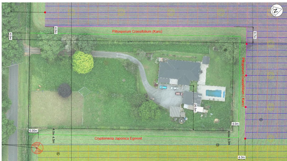
Figure 1: Amended site plan showing the type of planting along the boundaries, the setbacks, and the setbacks of the artificial kiwifruit shelters.
