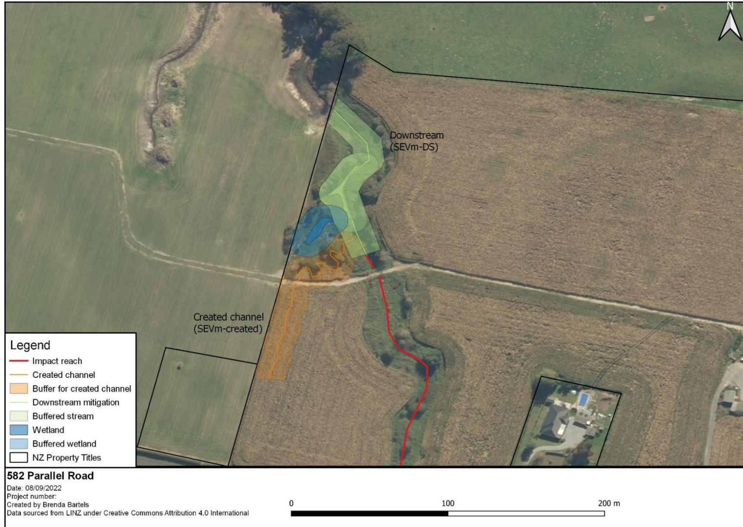
Figure 11: Option 2: Proposed mitigation showing a 10 m buffer. Downstream SEVm-DS also includes 115 m 2 of adjoining floodplain habitat and an additional wetland area. Orange area shows the indicative created channel and buffer.
