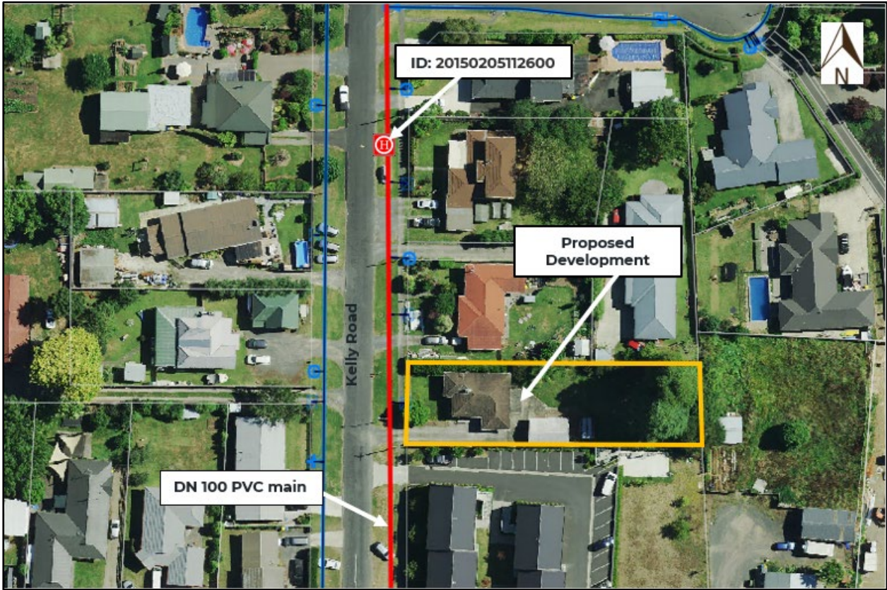
Figure 3: Overview of the water supply network
