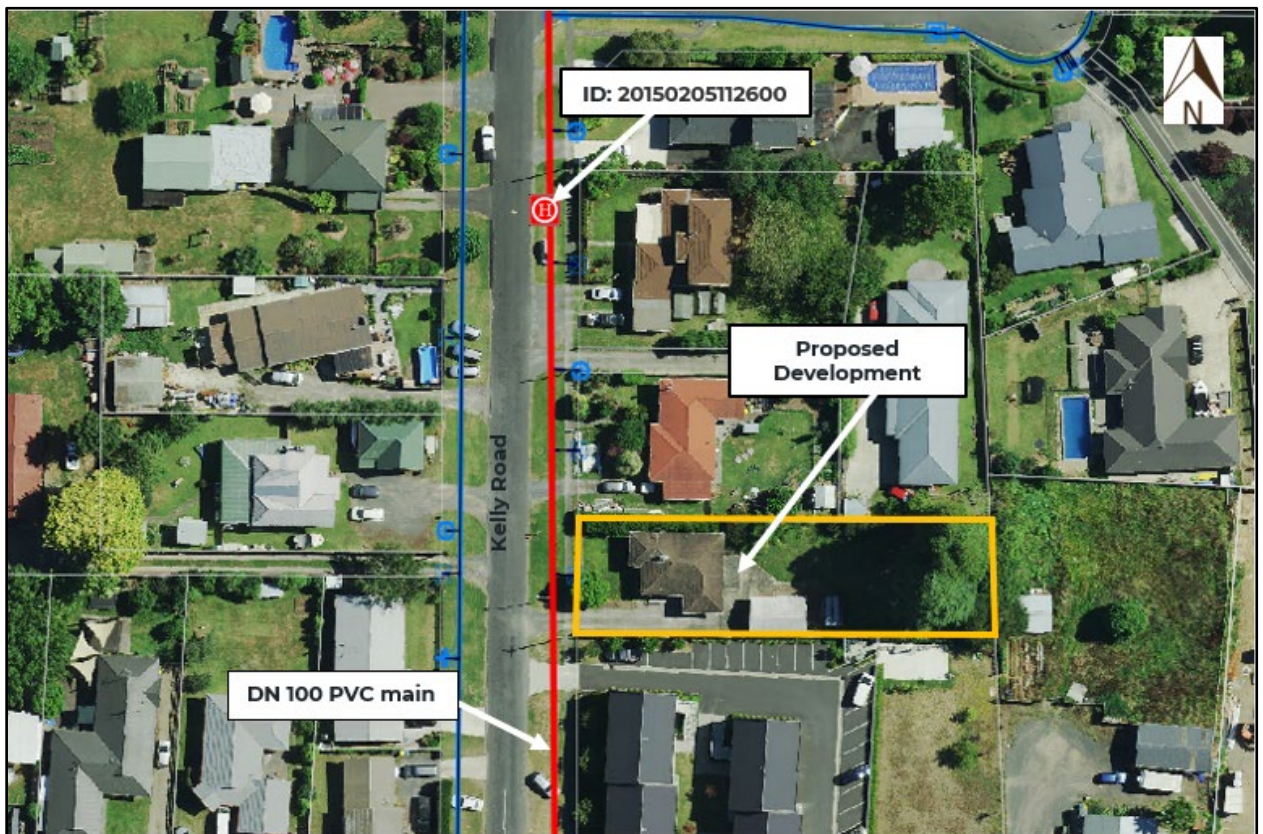
Figure 2: Overview of the water supply network
