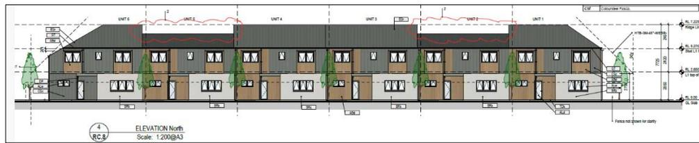
Figure 3: Updated northern elevation illustrating the stepped roof profile (sourced from Appendix 1, dated 27.02.2024).
