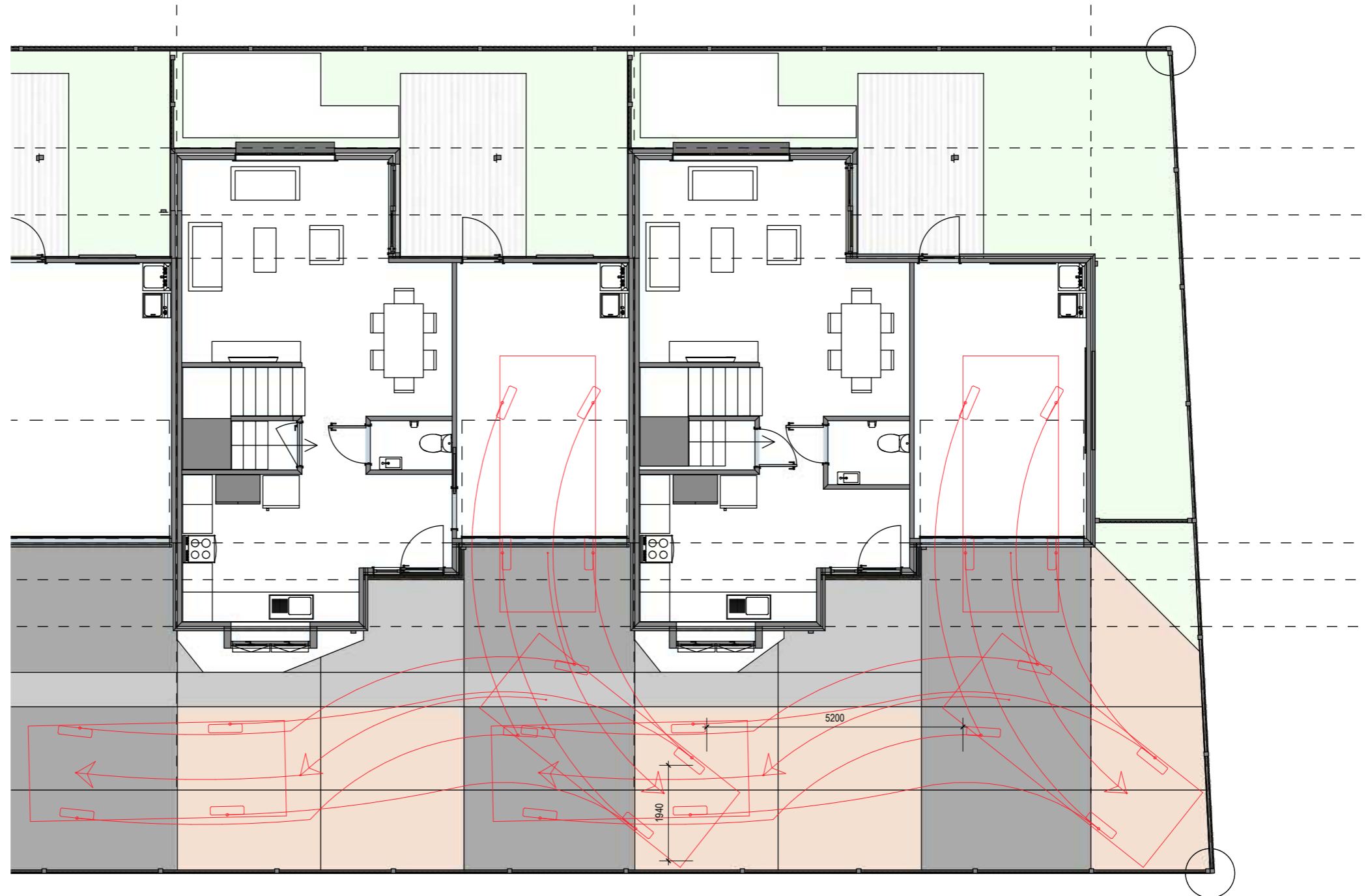
REVERSING MANOUVRE VEHICLE PATH OUT OF GARAGE TO AS/NZS 2890.1 B99 VEHICLE.
