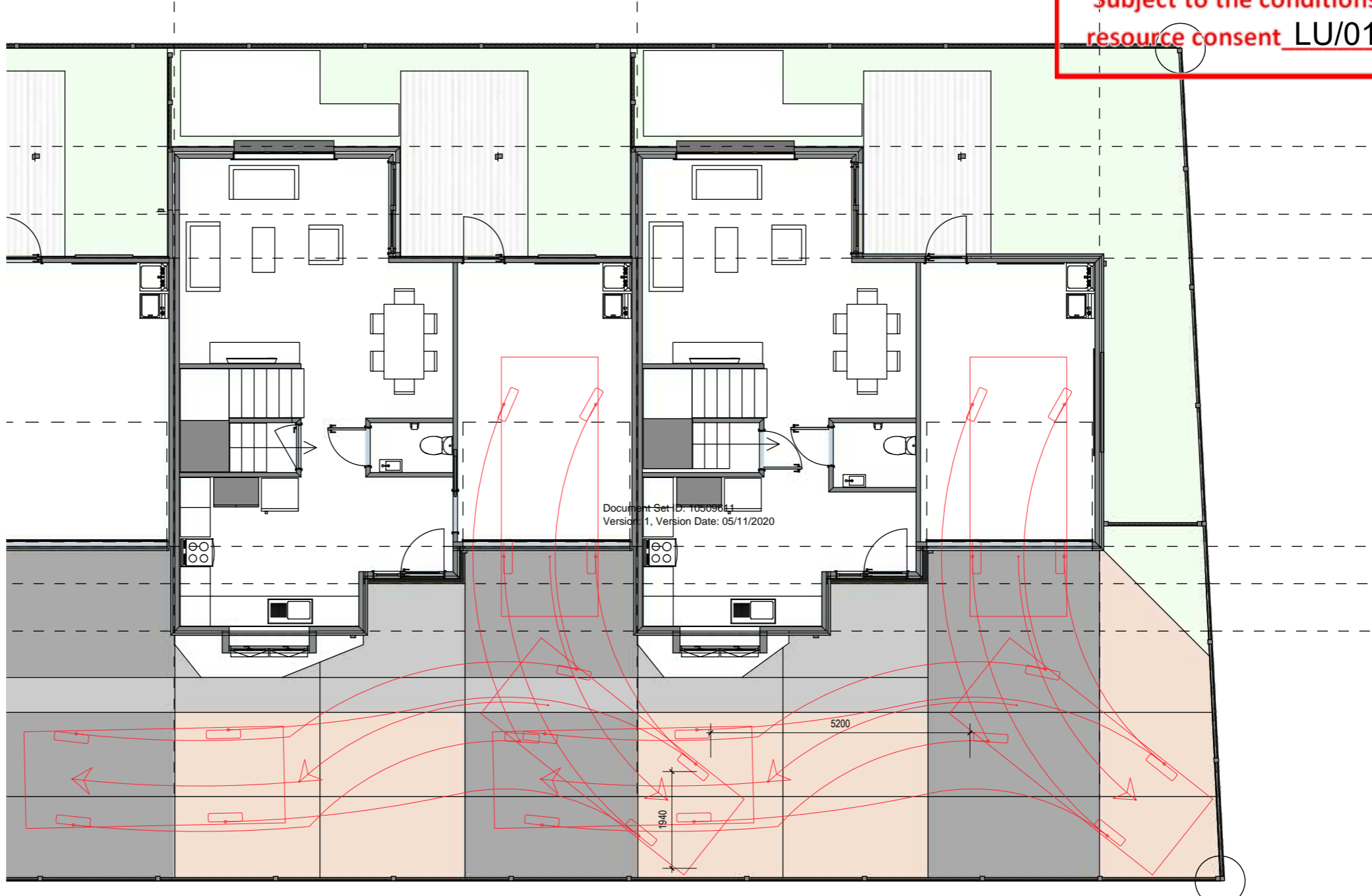
REVERSING MANOUVRE VEHICLE PATH OUT OF GARAGE TO AS/NZS 2890.1 B99 VEHICLE.
