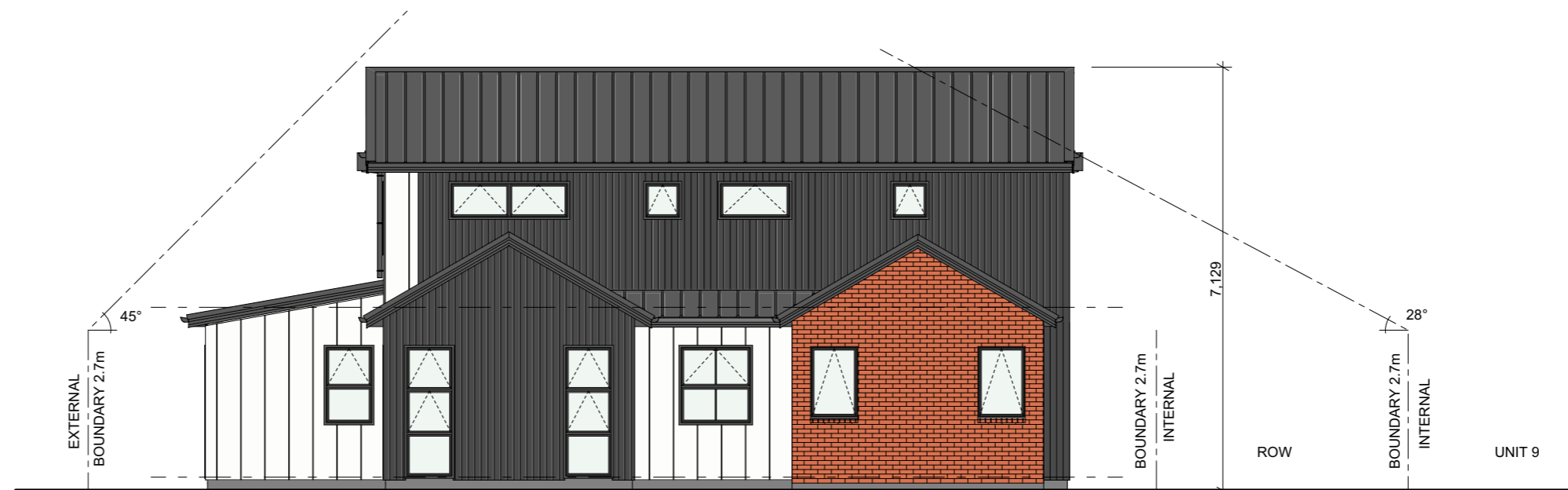
EAST ELEVATION - UNIT 7 & 8
