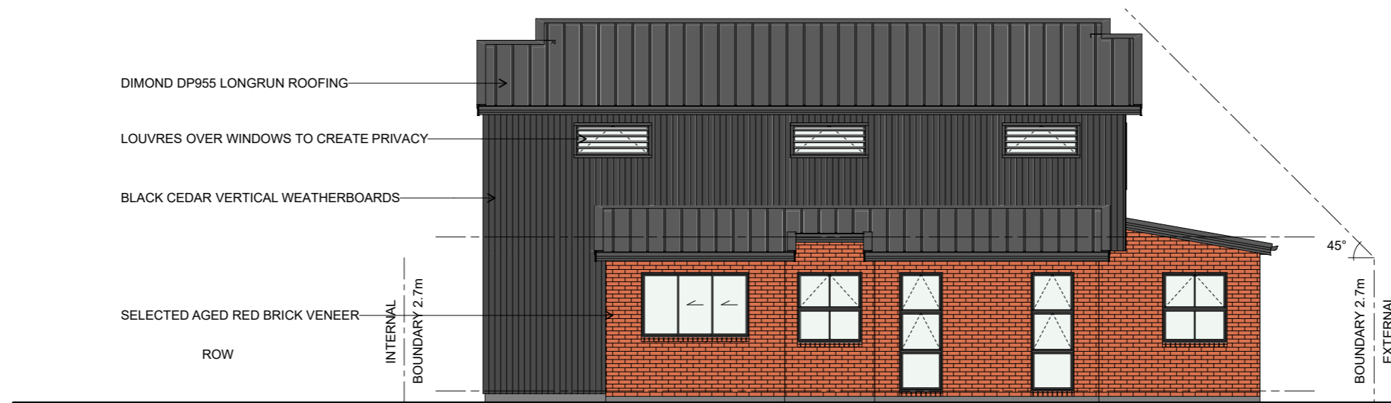
EAST ELEVATION - UNIT 5 & 6
