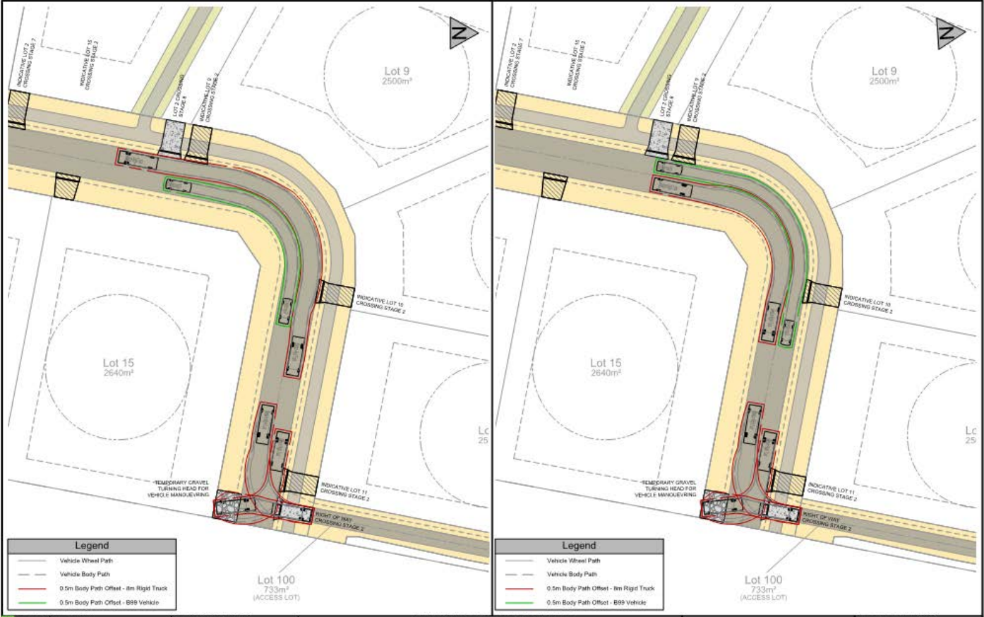
Figure 6: Vehicle tracking for a medium rigid truck (8m) and 99 percentile car
